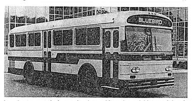
In order to meet the increasing demand for a dependable transit bus, in 1976 the Company introduced a pusher coach. This unit, with the power plant in the rear, meets a new need for transit and intercity buses. Like the forward control, both the chassis and body are built by Blue Bird to offer safe and dependable transportation.
