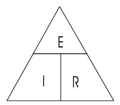
is the world's standard for following electrical circuits and without it we would not know how to figure wire size, or amperage or resistance and voltage and how they interact upon one another.
