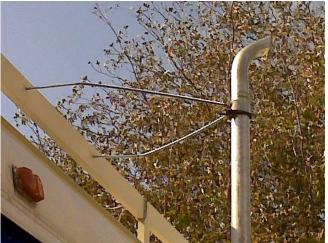
lower part of the plug used. The small inverter is resting in the closet out of the way and at the ready and with a strip of the looped side of Velcro, attaches solfumes high and into the winds, there by not being a bother, so much, to the neighbor. In the older Coaches, an aftermarket add on that can be mounted manually to the gent set exhaust, and some of those can be fairly expensive and with a little planning they can be inexpensive as well. Here is what a \$50.00 dollar bill did for us.
