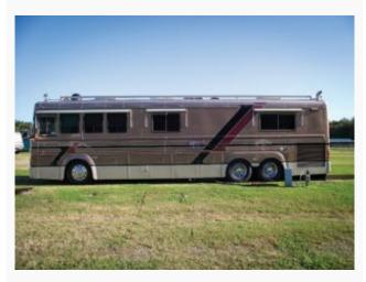
Stout construction materials include a 20-gauge steel roof, 14-gauge steel floor and 16-gauge steel side panels. The original exterior paint continues to shine.
