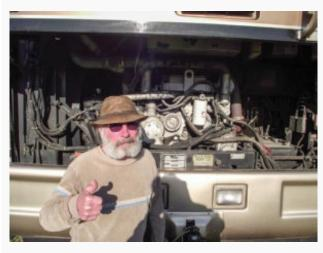
Darrell Beaton gives a thumbs-up to his turbocharged 450horsepower 8V92A Detroit Diesel engine.
